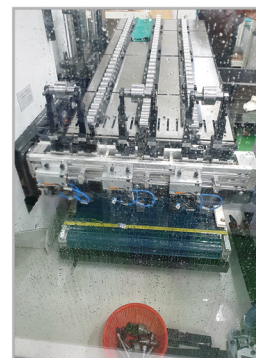
Multi-rail supply system
