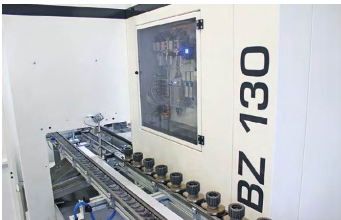
Workpiece storage as conveyor belt
