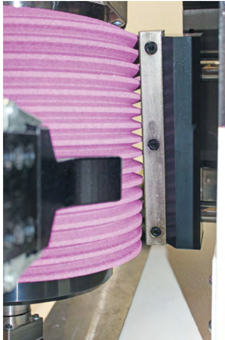
Patented OD-dressing and monitoring of the grinding wheel diameter
