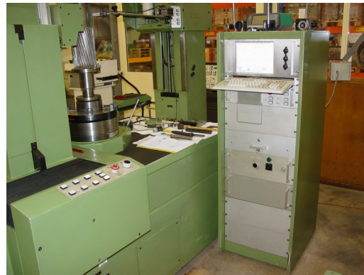
ES-41X Recorder 19" Unit with keyboard in a SP130
