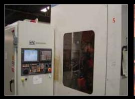
This machine was already a 5 axis hobbing machine, with one spindle. It was equipped with a proprietary Liebherr CNC which was very difficult to support. So we installed a new GE Fanuc 18i-MB CNC and GE Fanuc HVi digital servos and spindle drive for the owner.
