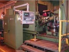
This Liebherr LC-1002 was in excellent mechanical condition, but the controls were very problematic. The old control was the proprietary Liebherr system, with little support or parts available. The controls we installed were GE Fanuc 18i-MB CNC with GE Fanuc Alpha HVi digital servos and spindle.
