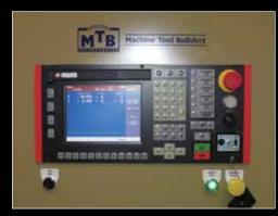
This hobbing machine was equipped with old East German controls that were unsupportable and no longer functional. MTB designed a replacement system around a NUM Axium Power CNC and Indramat Servos to control two axes of motion on this machine, and in the process gave the customer the ability to crown and taper hob as a bonus.
