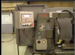
This hobbing machine was equipped with a relay control system that contained parts which were no longer available. MTB installed a small PLC, with HMI display to operate the machine. All the original machine systems were operated exactly like before, but now accessed through the HMI instead of a push button panel.
